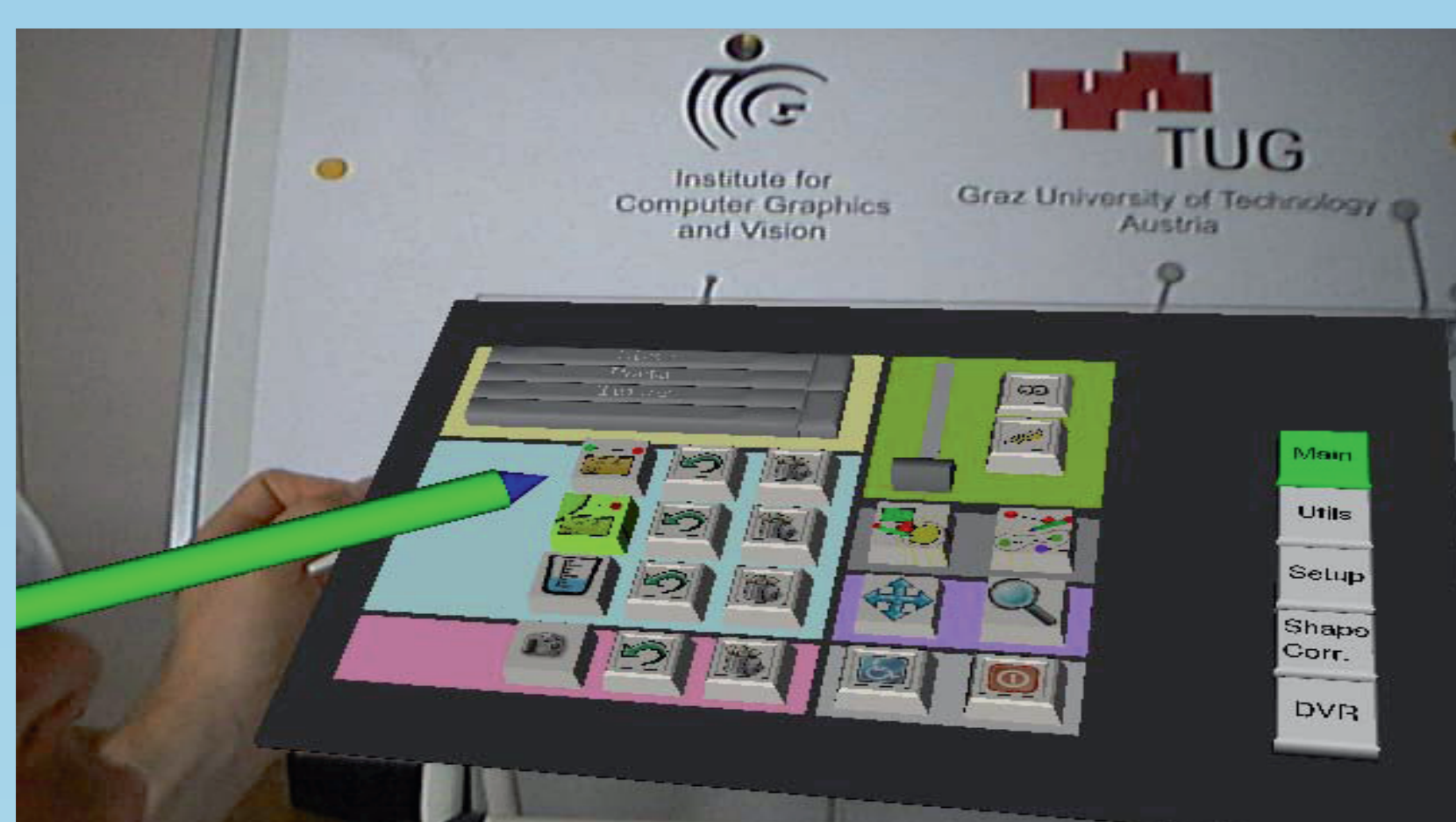
Fig. 3: The action button side of the PIP is shown – the pencil is used in order to activate the different functions.
